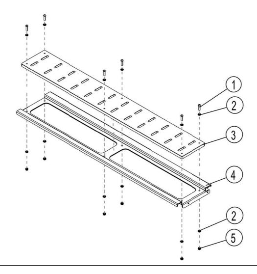
**(A)** Assemble the Wooden Shelf to the Frame as shown above and place a M6 Nut Cap over each Nyloc Nut once assembled.
