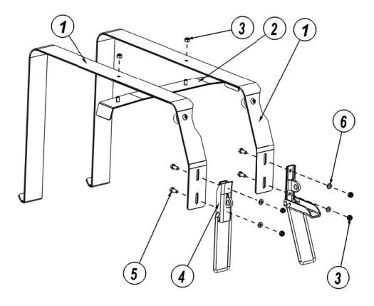
**NOTE:** Final adjustment of the latches must be done once the base is installed and the Jerry Can is inserted.
