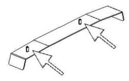
NOTE the 2 bolts on strap 2 (Item 2) are offset to one side. Make sure the shorter offset is to the left when assembling. See above diagram
