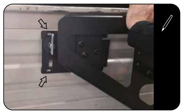
Loosely assemble Anti loose and Rubber stopper to the U-channel Plate.
