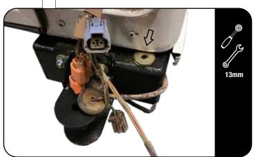
Loosely fit the box bracket with four M8x35 hex bolts, a M8x80 hex bolt, ten M8x19x1 washers and secure with five M8 Nyloc nuts.
