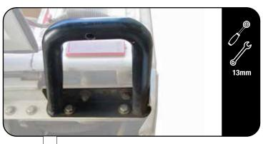
Remove the right hand foot step with a 13mm socket and wrench. Store this part in a safe place as you will not refit this part.
