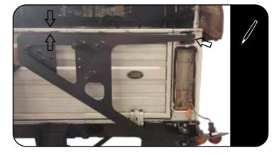
With the upper hinge (Item C) assembled to the swing arm and swing arm (Item B) attached to the Lower Hinge (Item E). Position the swing arm so that it is parallel with the tail gate.
