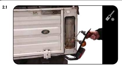
Remove right hand tail light assembly and disconect.
