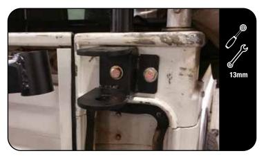
Fix and Secure with two M8x35 Hex Bolts, four M8 Flat Washers, and two M8 Nyloc Hex nuts. (Items 19, 7 & 6)
