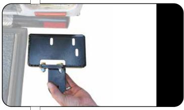
Take the box bracket (Item E in Figure 1.1) and lower hinge assembly, this will be fited to the vehicle in the orientation shown.
